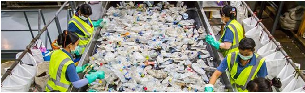
Figure 4 Sorting process of PET bottle wastes [12]
